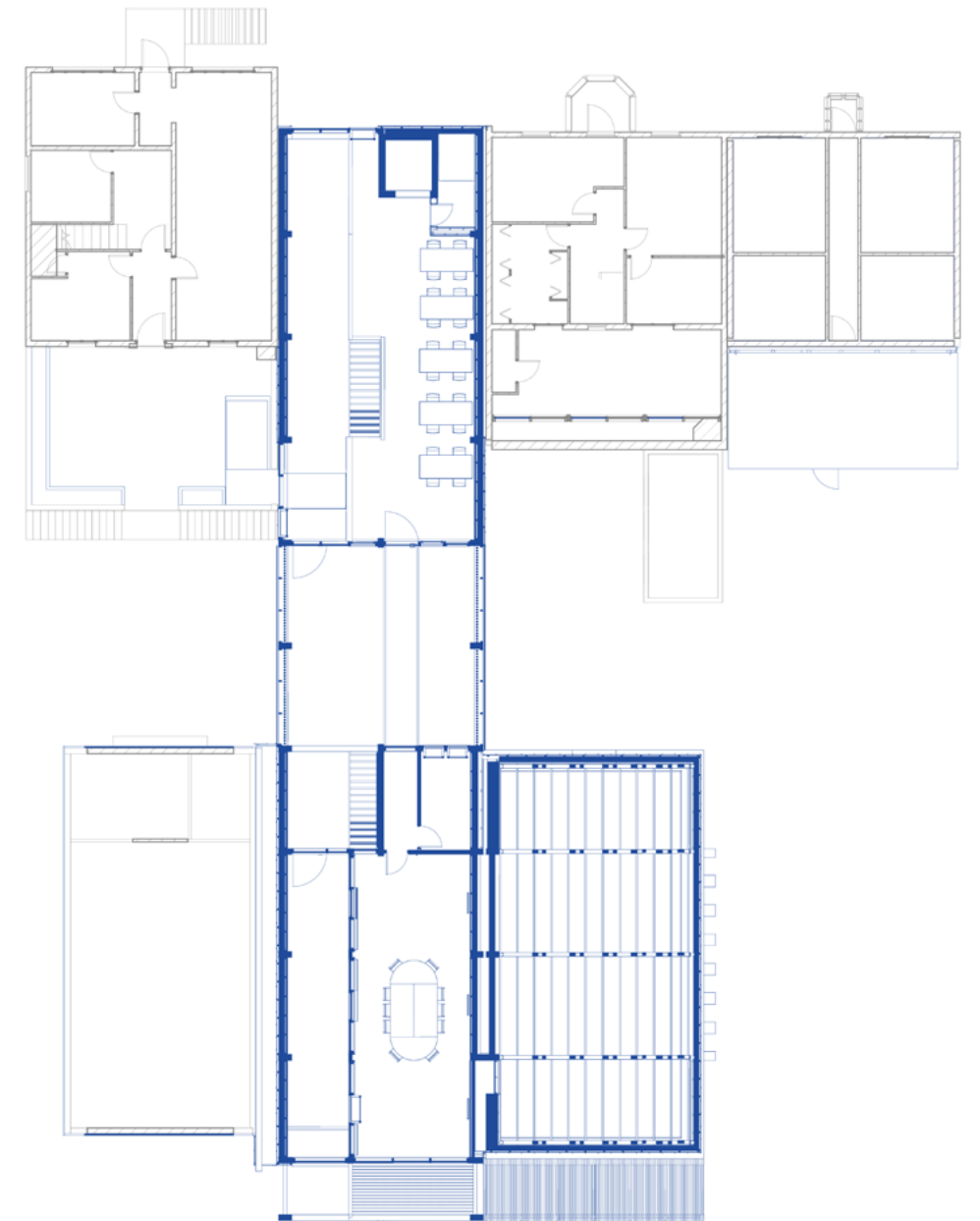
First floor plan — Existing (Gray) / Proposed (Blue)
